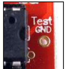
Ground Test Pad
